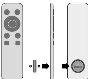
This product is delivered with a remote control that uses button-cell batteries. Please remove the batteries if the remote control is not in use for a long period of time. The buttons on the remote control match those on the control panel. The general functions and operating methods are the same.
